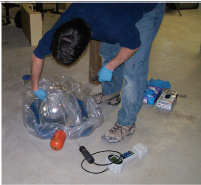
Seal testing for sub-slab vapor sampling
