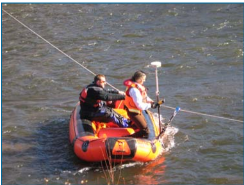
DEQ Environmental Science Specialist, Brian Bartkowiak (left), and TerraGraphics Engineer, Susan Firor (right), conduct a cross-section survey of the Clark Fork River in preparation for environmental remediation.
